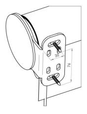
Start the screen roller blind installation to the ceiling by marking out the attachment holes of the supporting brackets.
